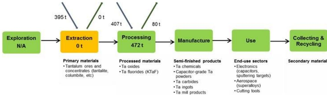
**Figure 471: Simplified value chain for tantalum for the EU, averaged over 2012-2016<sup>267</sup>**
