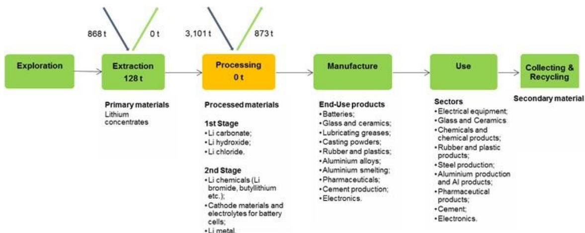
**Figure 165: Simplified value chain for lithium in the EU<sup>128</sup> (average 2012-2016)**
