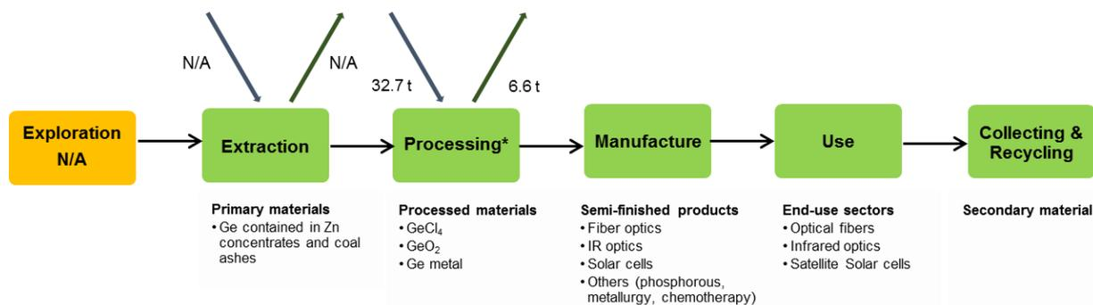
**Figure 139: Simplified value chain for germanium<sup>99</sup> for the EU, averaged over 2012-2016**
