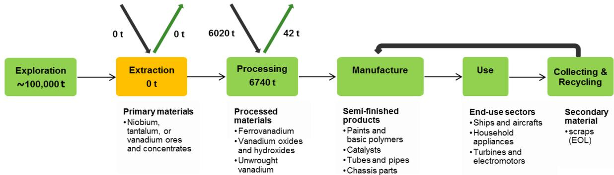
**Figure 500: Simplified value chain for vanadium in the EU<sup>287</sup>, 2012-2016**
