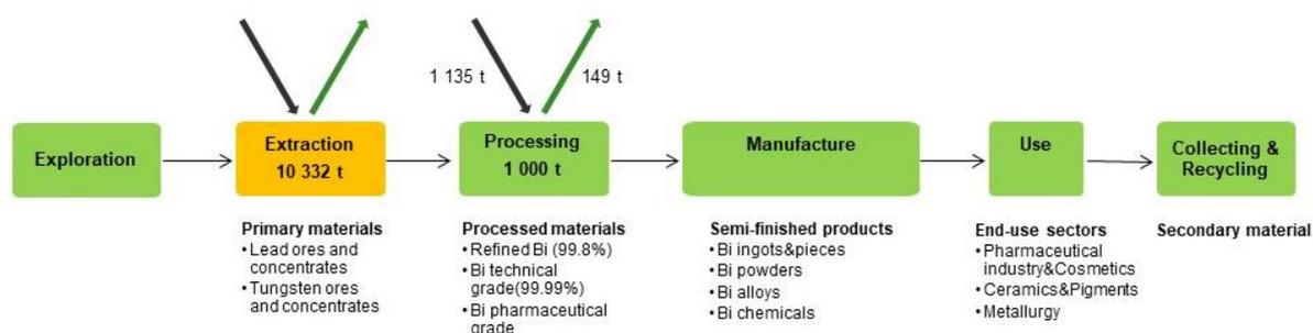
**Figure 61: Simplified value chain for Bismuth (2012-2016 average figures)<sup>33</sup>**
