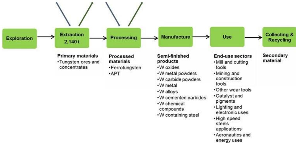
**Figure 487: Simplified value chain for tungsten for the EU, average 2012-2016<sup>281</sup>**
