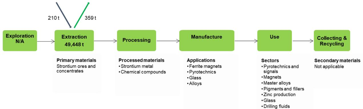
**Figure 464: Simplified value chain for Strontium for the EU<sup>264</sup>, average 2012-2016**
