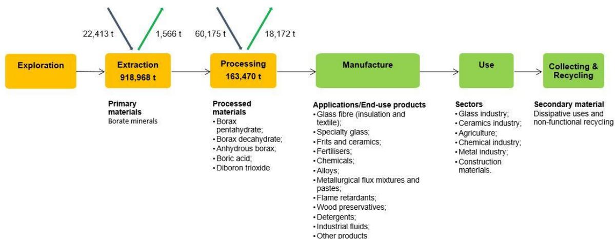
**Figure 70: Simplified value chain for borates for the EU, averaged over 2012-2016<sup>37</sup>**
