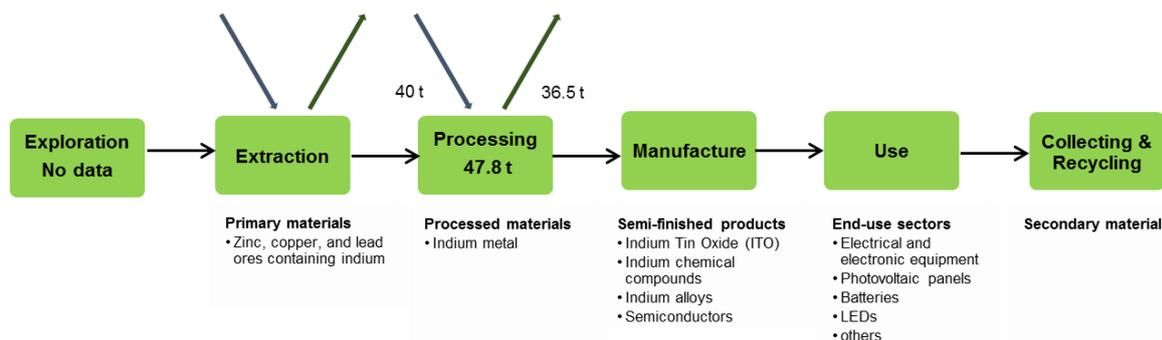
**Figure 156: Simplified value chain for indium, 2012-2016 for the EU, averaged over 2012 to 2016<sup>119</sup>**
