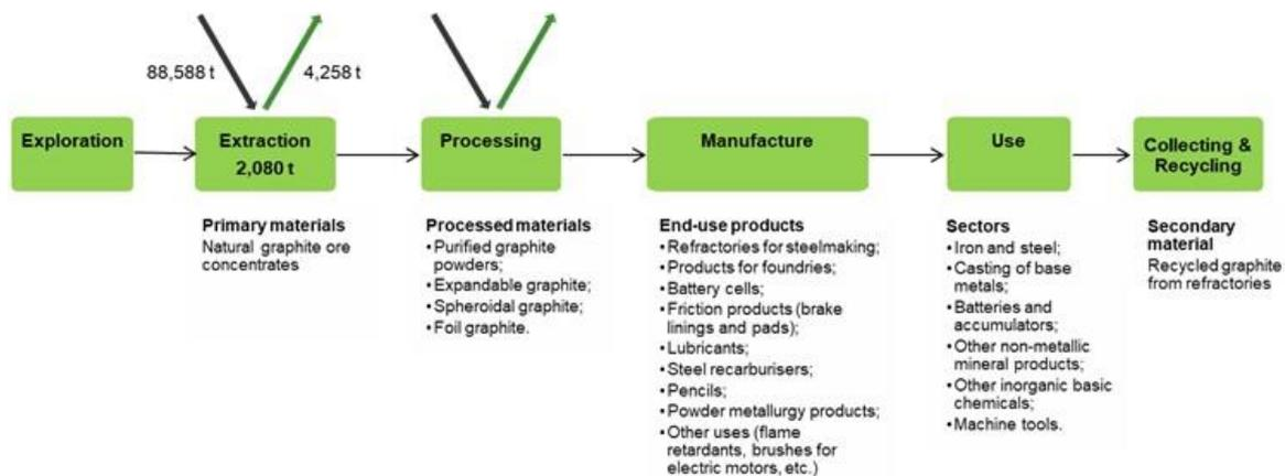
**Figure 193: Simplified value chain for natural graphite<sup>164</sup> (average 2012-2016)**
